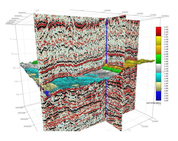
In advance of the upcoming drilling programs Discovery completed the Nike 3D survey (180 km<sup>2</sup>) on the southwest production trend acreage of PEL 512 and AVO analysis of surrounding 3D surveys covering the offset oil fields to the north and east of PEL 512.
